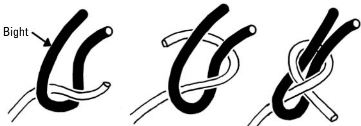
Figure 14-2: Tying a sheet bend.
